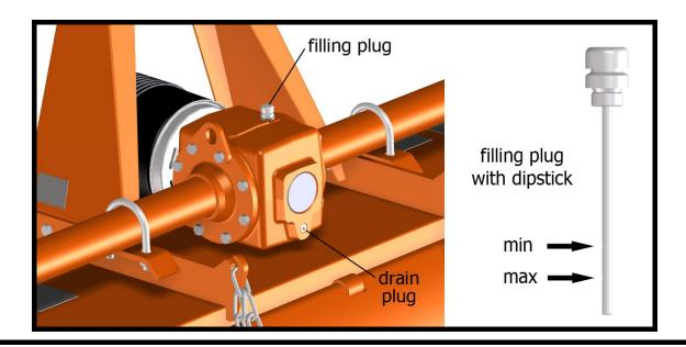
If the sign is below the minimum, fill up oil till restore the correct level.
