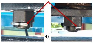
When split pin is removed, tighten the castle nut.
