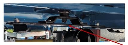
Remove M14x50 bolts from rotor bar/rotor bar holder assembly.
