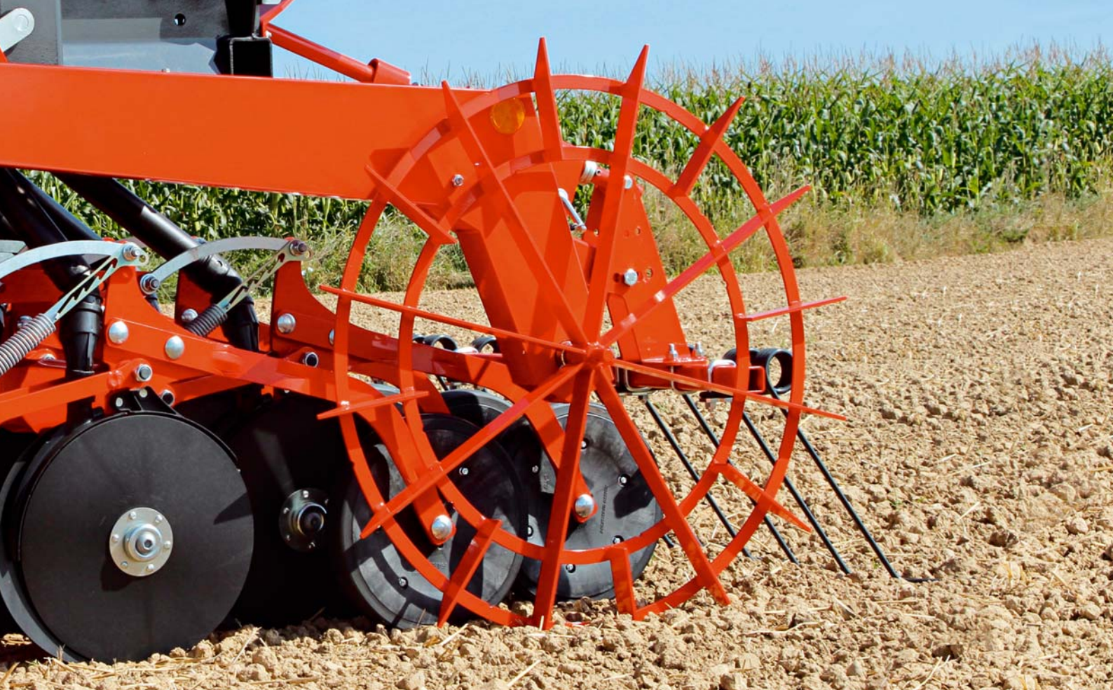
Covering the seeds and levelling the surface: a performing covering harrow
