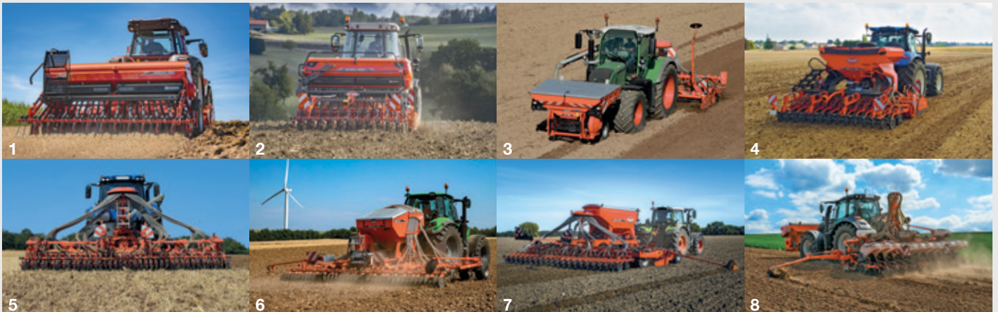
1. Mounted mechanical 2. Integrated mechanical 3. With front hopper 4. Integrated pneumatic 5. Foldable pneumatic 6. Mounted min-till 7. Trailed min-till 8. Precision seed drills.
