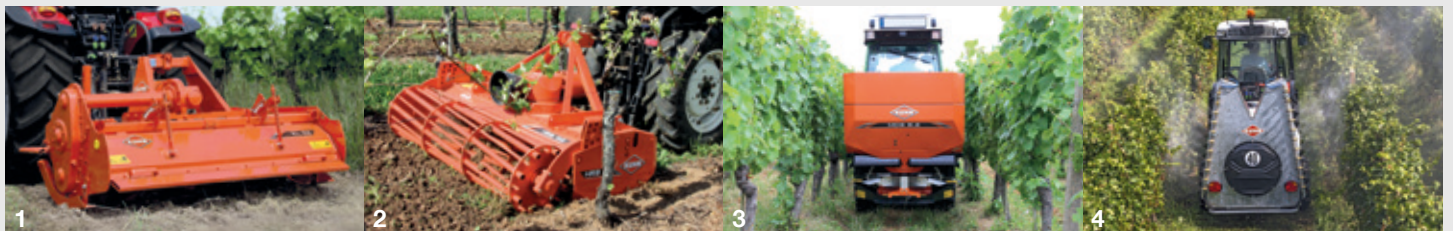
1. Power tiller - 2. Power harrow - 3. Fertiliser spreader - 4. Air-blast sprayer
