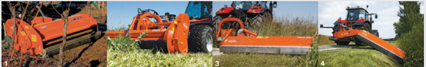
1. Vineyard and orchard shredders - 2. Front-mount landscape maintenance shredders - 3. Offset arm verge shredders 4. Professional-duty roadside mowers
