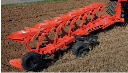
The wheel is equipped with a central pivot allowing it to automatically follow any changes in working width. The
