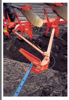
Available for the complete plough range the arm allows the use of a furrow press with easy hooking up and hydraulic push-off. On the pick-up hook part of the arm where there is most risk of damage all grease nipples and hydraulic hoses are protected inside the structure of the head. The arm folds up conveniently for subsequent transport.
