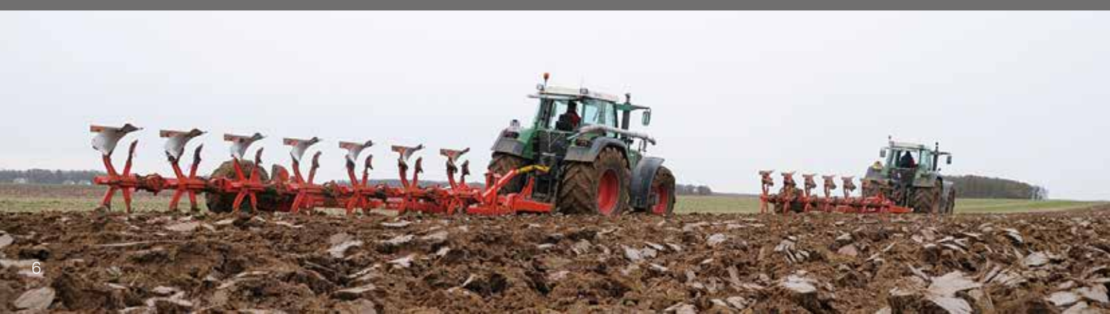
3. Offset : by mechanical tie rod or hydraulic cylinder (as an option) makes the inter-tyre adjustment from 1.15 to 1.60 m. A gauge visible from the tractor cab facilitates setting precision.
