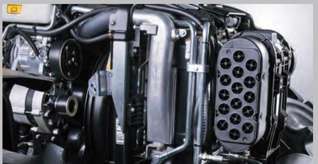
... as does the easy-to-clean cooling system with optional viscous fan.
