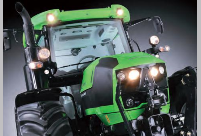
For optimal visibility during poor weather conditions. Eight working headlights in the roof and side posts. Two working headlights in the bonnet.
