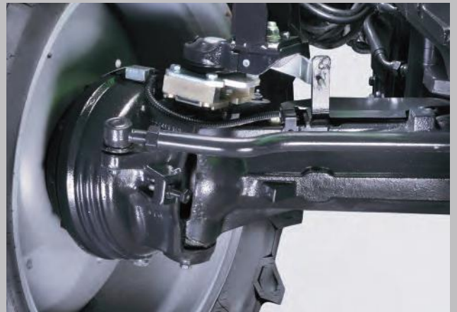
A unique safety concept from DEUTZ-FAHR. Separate oil cooled disc brakes in the front axle.
