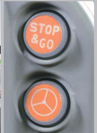
Front loader joystick with Powershift buttons, Stop&Go, SDD rapid steering system ...
