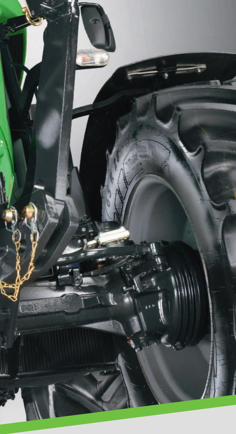
A unique safety concept from DEUTZ-FAHR. Separate oil cooled disc brakes in the front axle.
