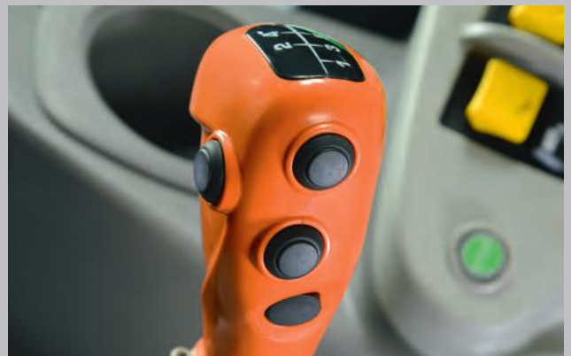
Comfort clutch and Powershift. Simply change gear at the push of a button without pressing the clutch.
