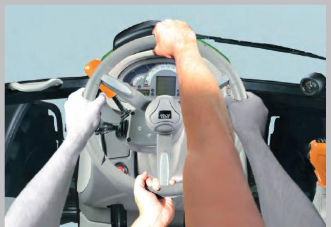
The SDD rapid steering system. Half the steering wheel rotation, double the steering power.
