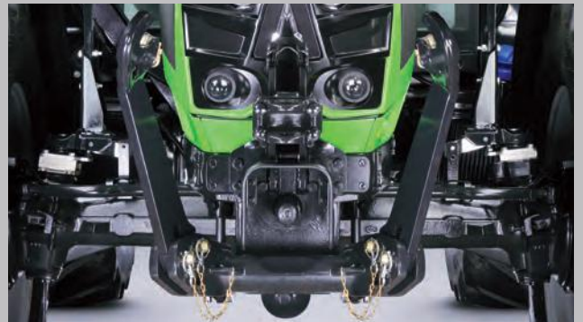
Front lift and PTO. Lifting capacity of 2,100 kg and 1,000 PTO.
