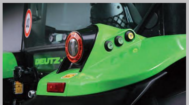
External PTO and hitch controls for straightforward equipment mounting and external equipment operation.
