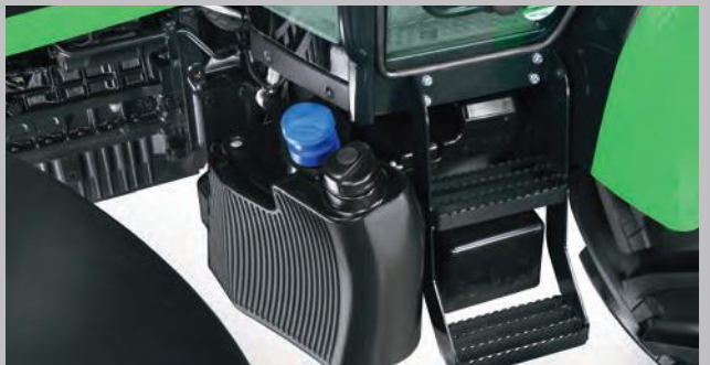
A fuel tank that holds up to 145 litres and 10 litres of AdBlue allows long working periods.(depending on model)
