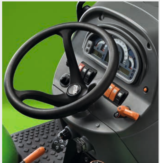
Engine speed memory. Save and recall an engine speed only by pressing a button.
