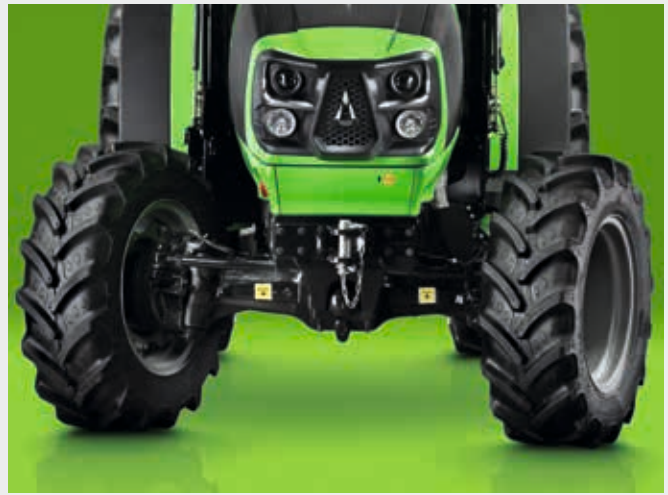
True 4-wheel braking thanks to front brakes.
