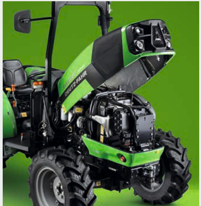
Easy to maintain thanks to wide opening single piece bonnet.
